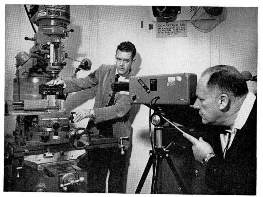
HOW WHITE IS WHITE? The colors used on Air Force instrument panels must be in accord with federal standards. Lee Sparks (1514), member ofthe project engineering group, and Hank Guttmann (1642) use a color photometer to determine whether a Sandia-designed display unit meets specifications for "lunar white." The test unit is mounted on a milling machine to permit precise positioning.
